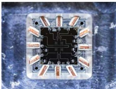
Top down view of the gmon qubit chip (0.6 cm x 0.6 cm) connected to microwave frequency control lines (copper) with thin wire bonds.
